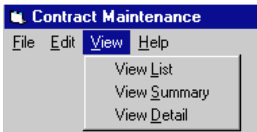
Figure 8.18 Don't start each drop-down menu item with the same word on the menu bar.
